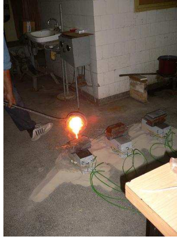
Fig.4. Mould casting of the liquid cast iron
