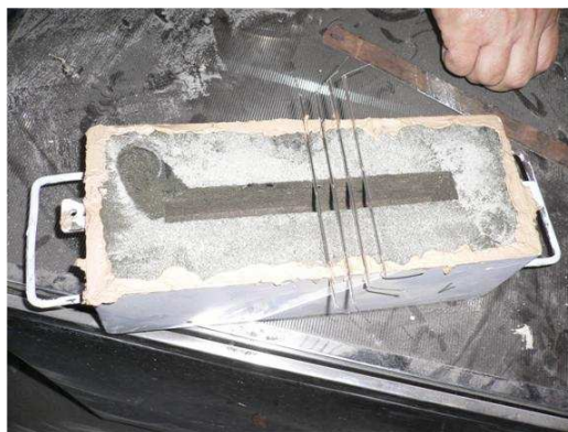
Fig. 3. Location of thermocouples on the mould during casting.
