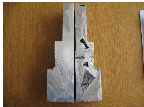
Figure 5. The position of shrike holes for the two casting variants: a) variant 1; b) variant 2
