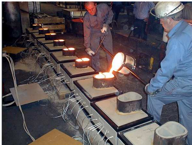
Figure 5: Practical experiments to follow the solidification pattern.
