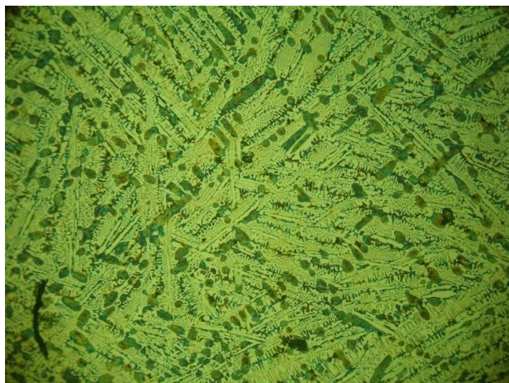
Fig. 4 – Structure of manufactured iron that was overheated in liquid state at temperature of about 1,500°C. X 128 (sample processed by chemical reactive).
