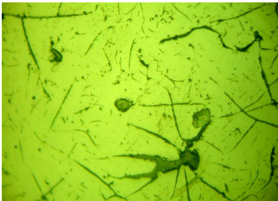
Fig. 1 – Structure of grey pig iron used for manufacture. X 48,8 (sample unprocessed by chemical reactive).
