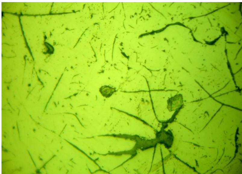
Fig. 2 – Structure of pig iron used in charge of the furnace. X 48.8.
