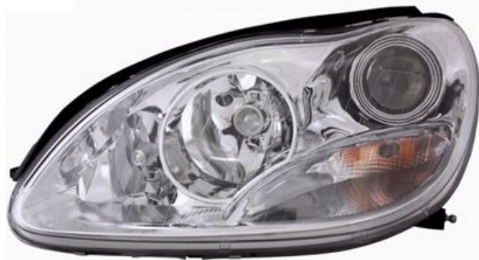
Fig. 1 – Lens welded on the housing – automotive lamp.
