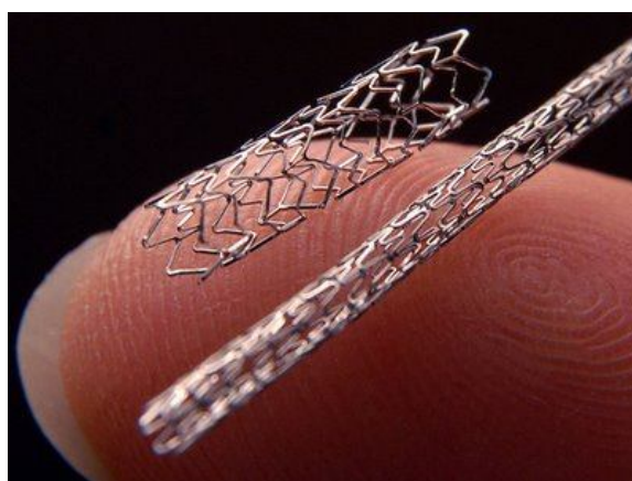
Fig. 1 – Coronary stent made of biodegradable metallic material.
