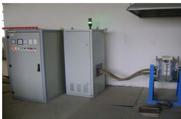
Fig. 1 – Induction heating furnace of medium frequency 8,000 Hz.
