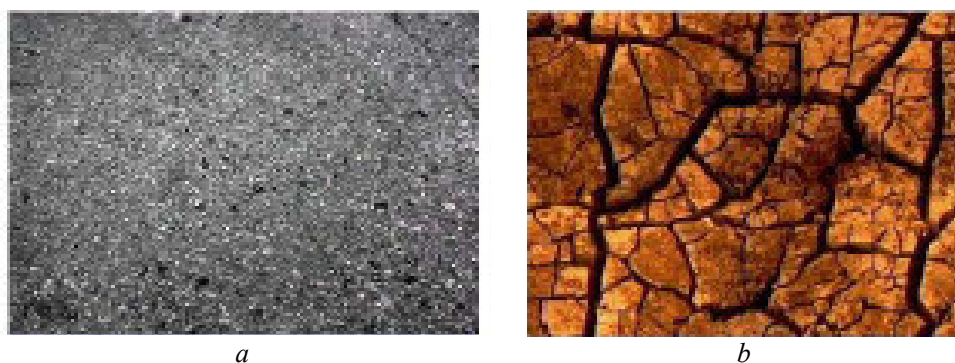
Fig. 1 – Composites used in dentistry (Gregory et al. , 1992): a – dental composites reinforcing macro-particles can degrade easily and are more difficult to polishing; b – dental composite reinforced with micro-particles in excess are viscous and difficult to model.
