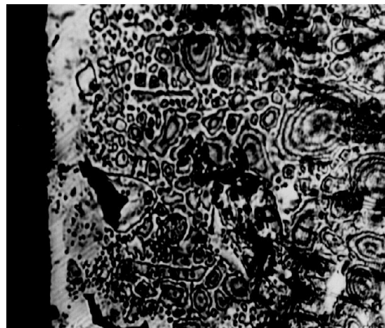
Photo 5. Sample microstructure nr.3, after treatment of 1150 0 C, temperature (x200).
