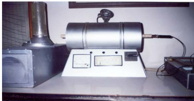
Fig.1 Equipment for the determination of fluidized beds cooling characteristics
