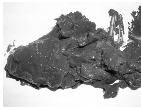
Fig. 4 Slam assay taked from settling tank after separation
