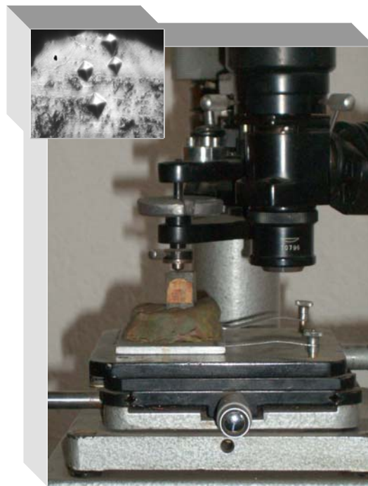
Fig.6. Apparatus PMT3 for microhardness measurements
