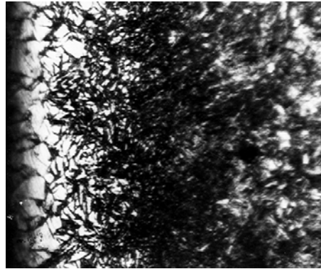
Figure 8. Microstructure of steel 40Cr10 nitrated ( T_d = 750^\circ\text{C} ; t_d = 6 min) cooled at 600^\circ\text{C} and chilled at 800^\circ\text{C} in electrolytic plasma ( T_{\text{aust}} = 750^\circ\text{C} ) - specimen J: nitro martensite + \underline{A}_{\text{rez}}
