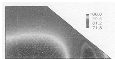
Fig. 3. Streamlines with contours of normalised mass fraction oxygen % ( 100 \times W_0 / 0.22 ), V_{in} = 1.0 \times 10^{-4} , q_l = 0.5 q_{L,0} , K = 5 \times 10^{-10}
