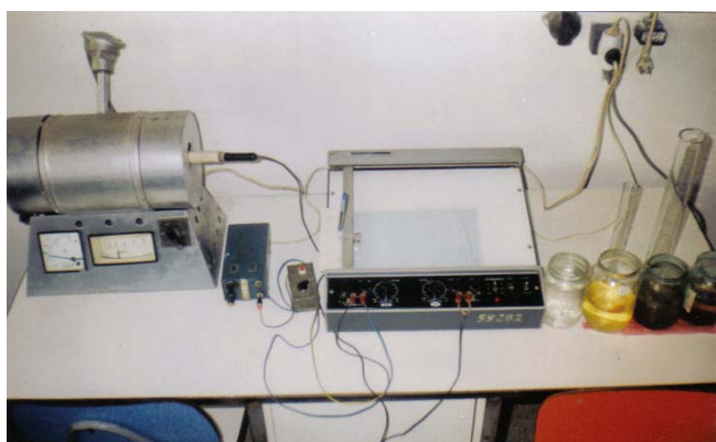
Figure 2. Experimental installation used for cooling curves determination
