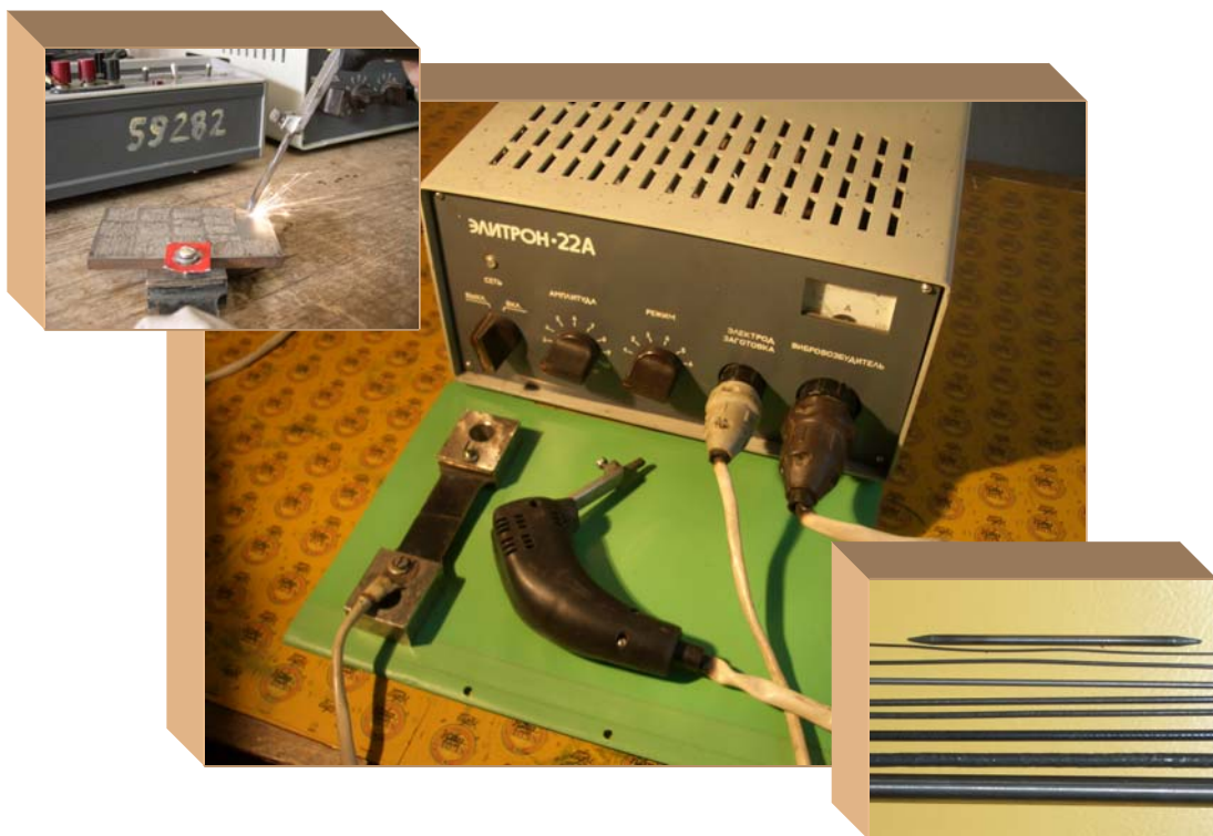
Fig.4. Elitron 22 –the installation for sputtering deposition with different kind of electrodes
