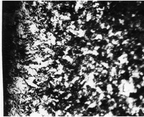
Figure 6. Microstructure of steel 40Cr10 nitrated ( T_d = 700^\circ\text{C} ; t_d = 6 \text{ min} ) and chilled from 750°C in electrolytic plasma, followed by tempering ( T_{inc} = 550^\circ\text{C} ; t = 1h ) – the exterior layer of specimen 3I: \underline{M}_{rev} + nitrides + carbides
