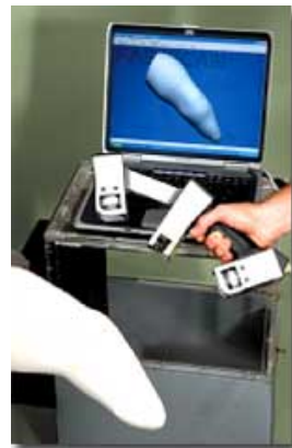
Fig. 4 The scanner used in BioSculptor system
