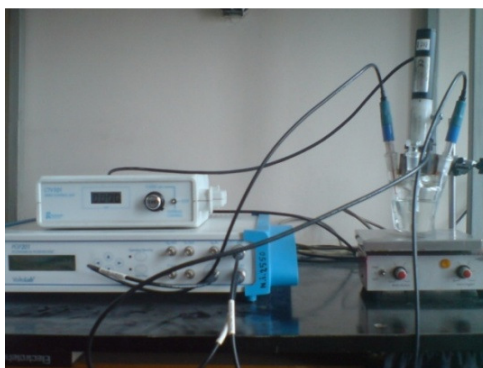
Fig. 2 – Potentiostat equipment used in electro corrosion tests.
