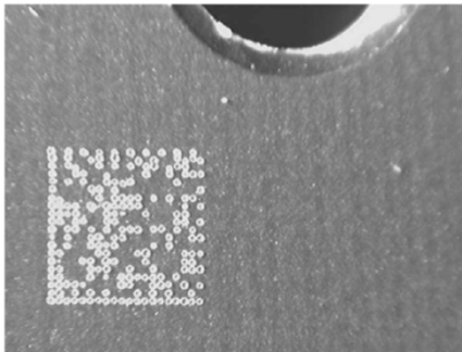
Fig. 9 – 2mm square data matrix code containing 26 alphanumeric characters directly marked onto a printed circuit board marked with a 5W CO 2 laser beam and a 115 micrometer spot size, 0.38ms -1 .
