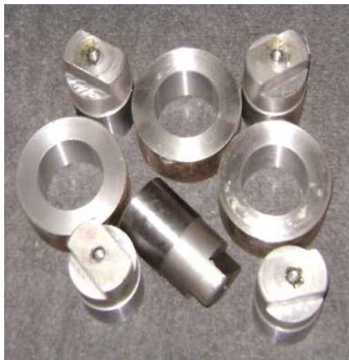
Fig. 2 – Parts ready for assembly with shrink.
