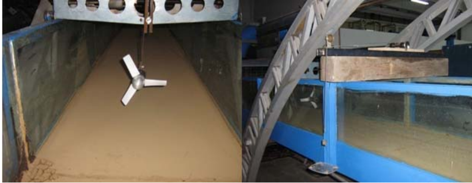
Fig. 2 – The experimental miniturbine located in the channel.
