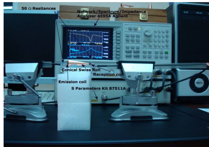
Fig. 2 – The equipment for measurement S parameters.
