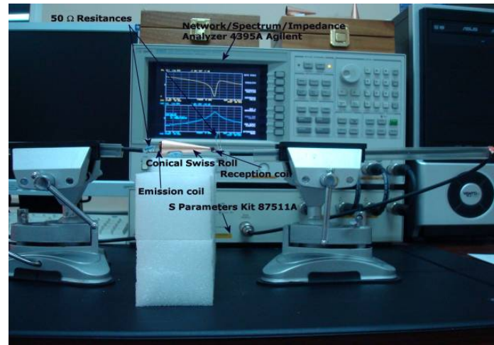
Fig. 2 – The equipment for measurement S parameters.
