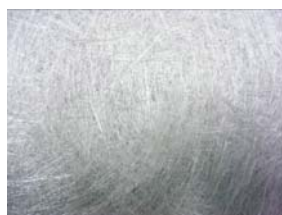
Fiberglass - short fibres (MAT)
