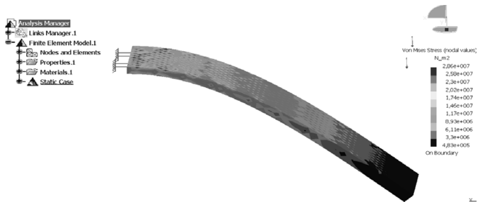
Fig. 3 – Concentrated load (10N) 1000g.
