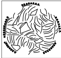
Fig. 4 – Drawing of a crystalline body at the beginning of the solidification range, when there is less remanent F_j ; • – inoculating agent atoms.
