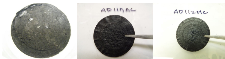
Fig. 2 – Buckypapers non-cleaned, acetone-cleaned, and methanol-cleaned from left.
