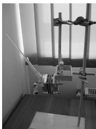
Fig. 3 – Experimental stand for resistance to permeation.
