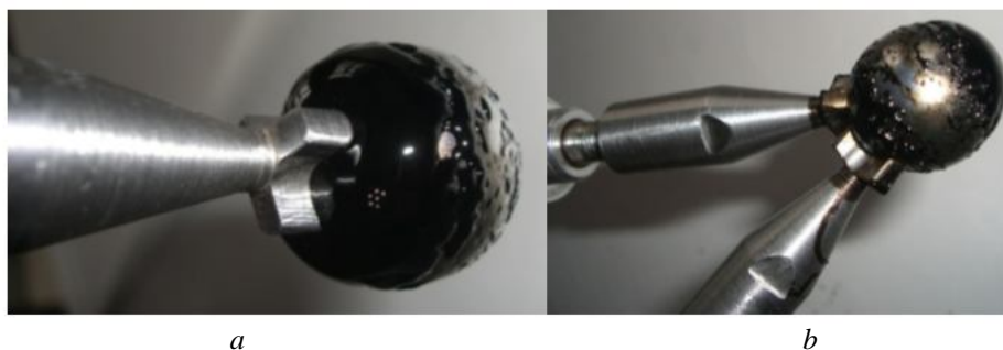
Fig. 10 – Magnetic sphere interaction with the support surface of the shanks in the presence of ferrofluid: a – shank at the pole of the magnetic sphere; b – location of two shanks at the sphere pole.
