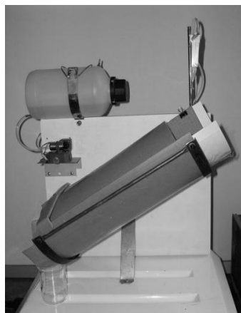
Fig. 1 – Experimental stand for resistance to penetration by liquids materials.
