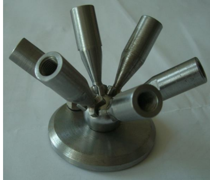
Fig. 11 – Positioning of six shanks of the joints on the magnetic sphere fixed on the vacuum-aerostatic support.
