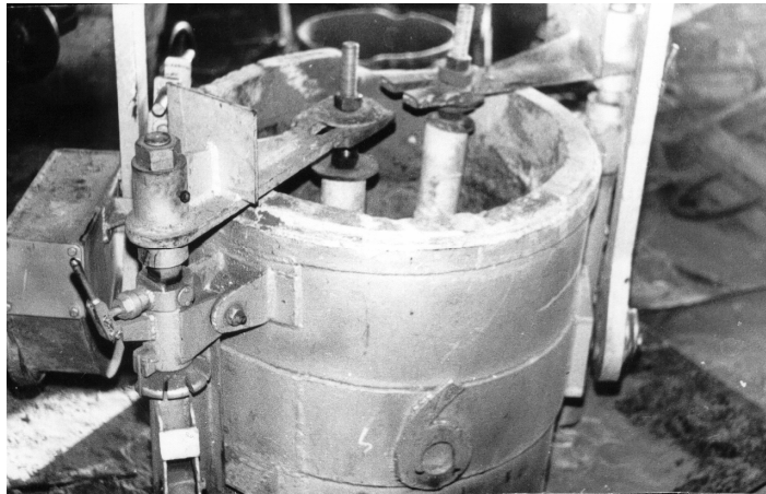
Fig. 4. The inoculant ladle achieved and used for experiments (with two stoppers placed equidistantly and two inoculant chambers).
