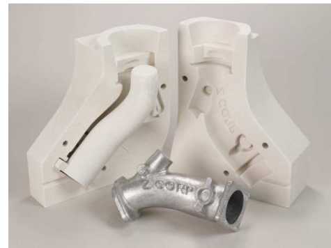
The mold to produce a cast metal part
