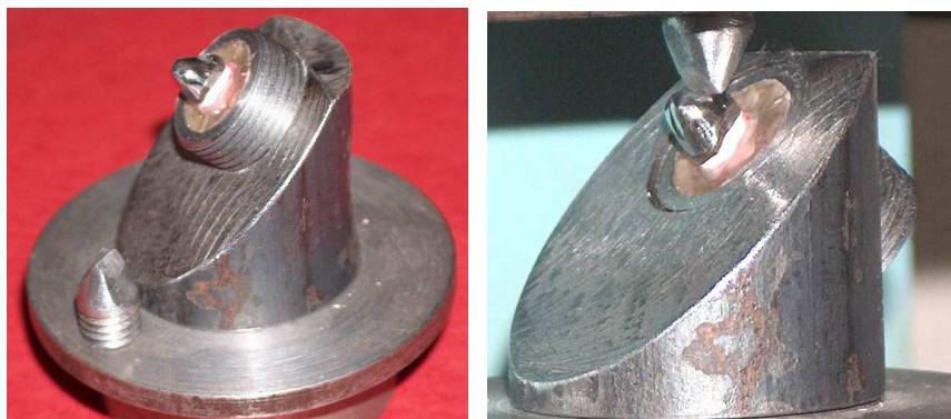
Figure 6. a)The specimen mounted in the testing device;
