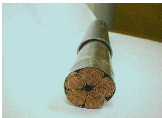
Fig.2. Super conductor cable from ITER
