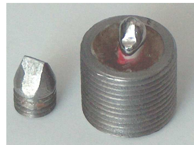
Figure 5. The specimen mounted in metallic cylinders
