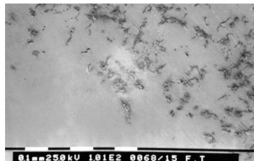
Fig.5. Quasillamellar graphite separation or star of the bimetallic plate (SEM x 100)
