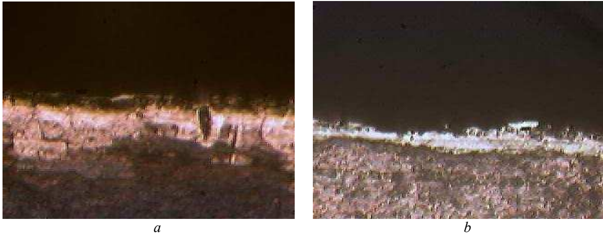
Fig 3. Structural microphotography for copper samples sparking with platinum electrode: a) regime II; b) regime III; attack with 20% ferric chloride; 1x400; 1x200.
