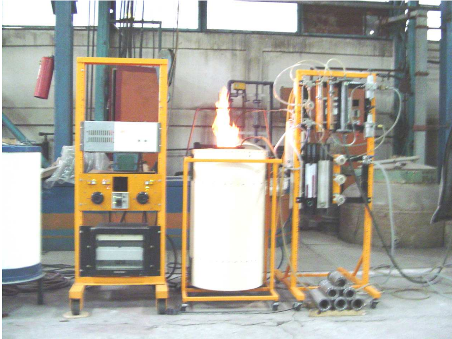
Figure 2. Image with nitriding furnace.
