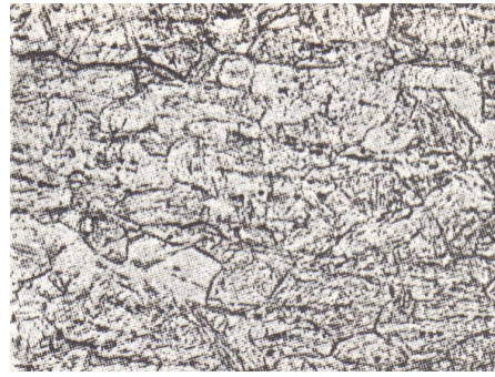
400:1 Fig. 4 Steel hardened and deformed with 25% degree. Vilella attack
