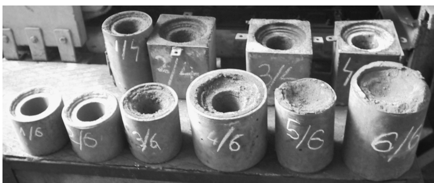
Fig. 3. Die aspect with refractory batch of slag and dross binded with furan resin (3/6.... 6/6) and sodium silicate ( 1/4 .... 4/4 ). (Unwashed dross)
