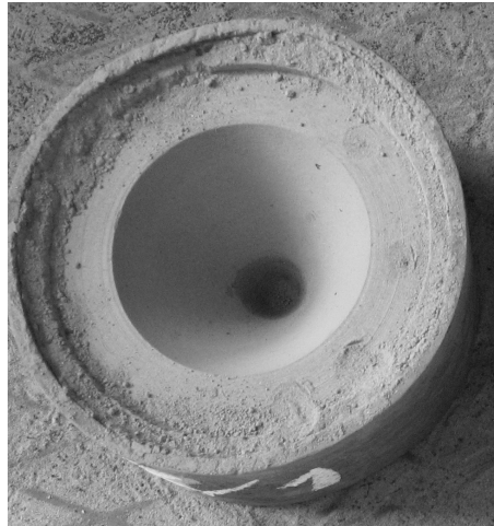
Fig. 4. Die aspect with batch dross binded with resin after 48 hours from execution (Washed dross)
