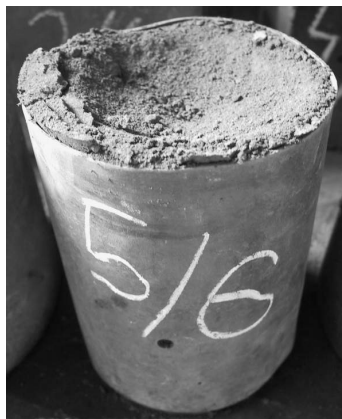
Fig. 5. Die aspect with batch binded with resin after 48 hours from execution (Unwashed dross)
