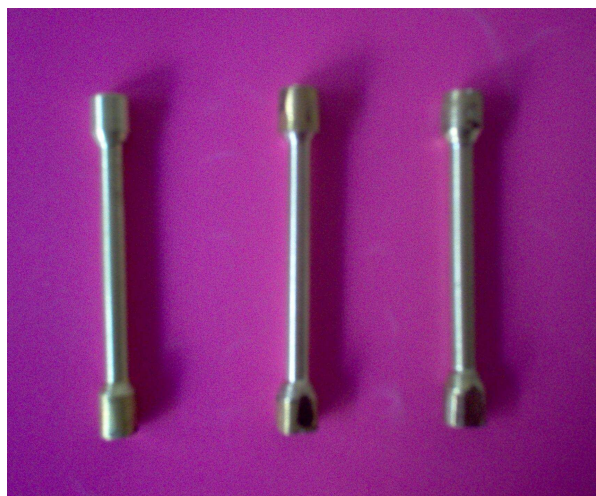
Figure 1. Standard sample, CuZnAl shape memory Alloys, for thermal fatigue test
