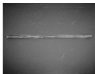
Fig. 6 – Hot-forged specimen (850 - 900°C).
