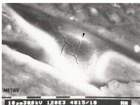
Fig. 5 – SEM microstructure revealed that "centers of corrosion" bands formed on the surface of ultrarapidly solidified alloy of nanocrystalline structure.
