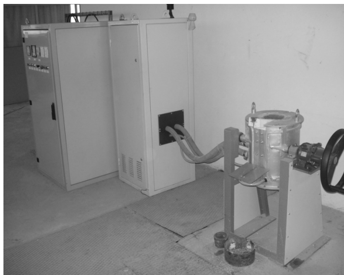
Fig. 3 – Induction furnace used for melting the alloy.
