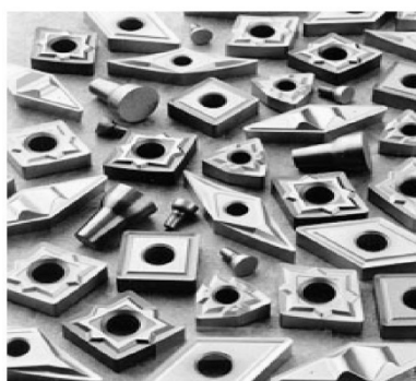
Fig. 4 – Assortment of cemented carbide inserts for use by different cutting tools.
