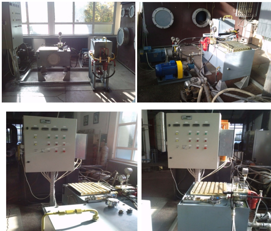
Fig. 2 – Adaptive hydraulic transmission for horizontal axis wind turbines for low power.
