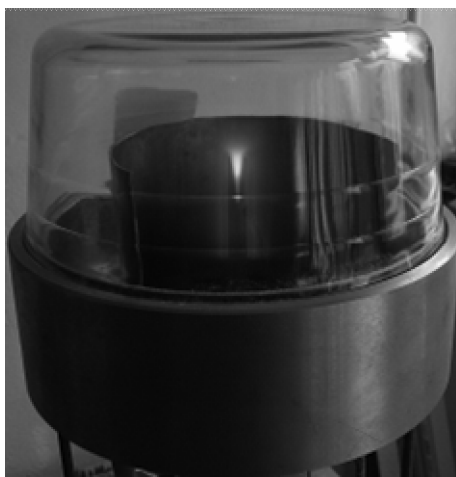
Fig. 3 – Plasma nitriding chamber with cathode grid.
