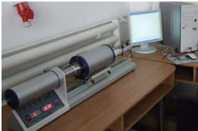
Figure 1. Dilatometer L75 with most important parts: command panel, heating oven and measurement head, data acquisition system connected to PC.
