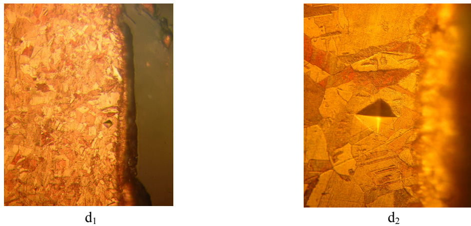
Fig.5. The microstructure of the weld accomplished by plastic deformation assisted by diffusion d , with fine polyedric recrystallized copper grains ( d_1 - \times 250 ; d_2 - \times 800 ).
