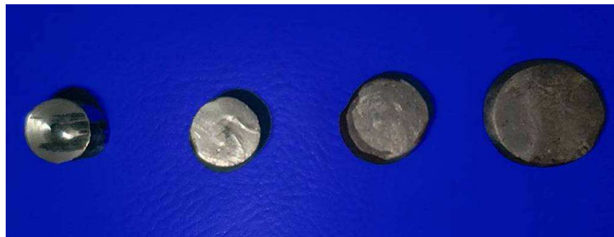
Fig.5 Deformed samples-up view a) Test bar, b) \epsilon=25\% , c) \epsilon=50\% , d) \epsilon=75\%
