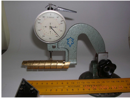
Fig.5 Initial shape and dimensions of the spring after forming and quenching heat treatment (850°C/ 15 min/ water) Fig.6 Training procedure of the spring, with controlled force application on Heckert FPZ100/1-type tensile testing machine: (a) initial shape of the spring; (b) deformed shape of the spring after about 15 cycles
