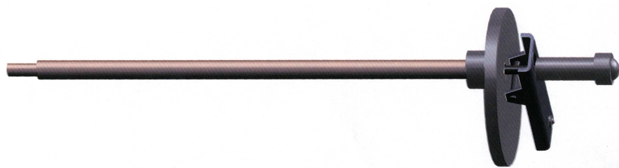
Fig. 3. The sensing element of the Invar thermostat for industrial applications
