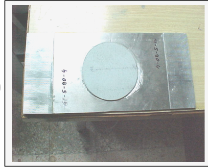
Fig. 4 – Experimental panel repaired by the composite patch method.
