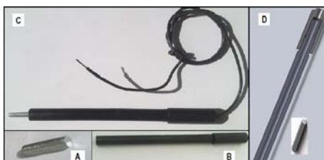
Fig. 5 – Antimony electrode; A- sensible element, B- plastic support for electrode, C- Antimony electrode assembly, D- Section through the body and an cap of electrode.
