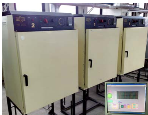
Fig. 1 – Oven-controlled system using LabView virtual instrumentation program.
