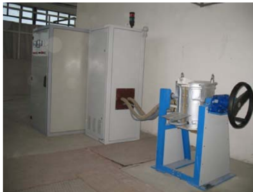
Fig. 9 – Induction melting furnace.
