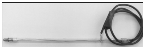
Fig. 6 – Antimony electrode with glass support.
