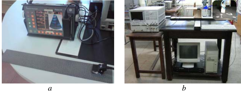
Fig. 3 – Nondestructive testing equipment: a – Ultrasound testing using phased array transducer and the equipment Phasor XS GE –USA; b – Eddy current testing using the transducer with orthogonal coils coupled at Network/Spectrum/Impedance Analyzer 4395A Agilent USA.
