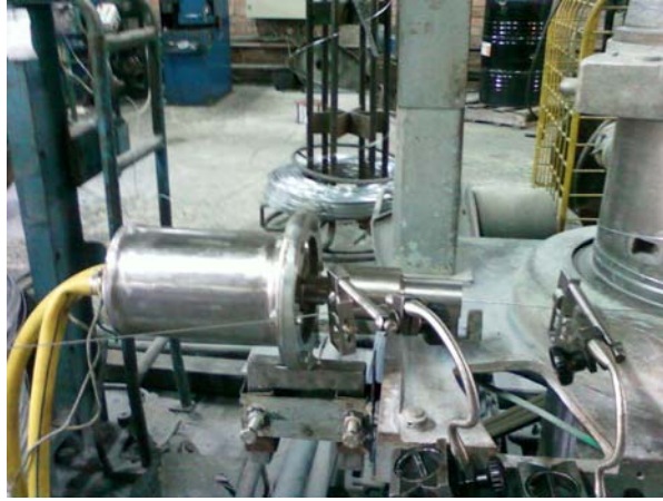
Fig. 1 – Photo of the drawing equipment UDZSA TO631 type, the reels area – based on the singular drawing principle.
