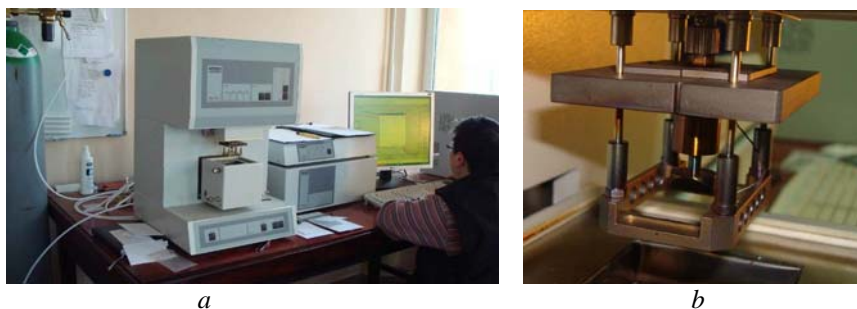
Fig. 2 – Dynamical Mechanical Analyzer: a – the equipment; b – three points bending fixture.
