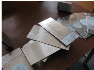
Fig. 1 –Experimental device for studying the interaction of Lamb wave modes. Piezo-MEMS (wafer transducers) positioning on the test panel bonded with composite patch to definitive the amplacement and frquency sensor.
