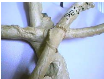
Fig. 2 – A-type cable at the first sampling during the pressurised oxygen ageing experiment (100°C și 4 bar).
