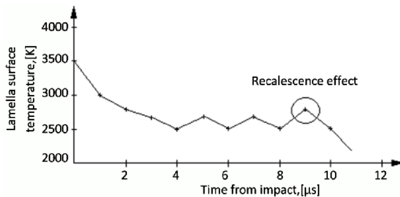
Fig. 2 – The evolution of front temperature solidification of a niobium splat, arc plasma sprayed using powder having a particle size of 22.5 μm.
