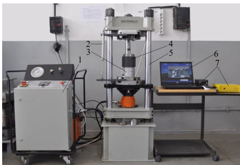
Fig. 1 – General view of the deformation installation: 1 – hydraulic unit; 2 – displacement transducer; 3 – load cell; 4 – deformation–extraction device; 5 – hydraulic press; 6 – notebook; 7 – Traveler 1 system.
