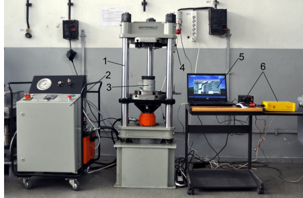
Fig. 2 – General view of the installation for the determination of the yield stress: 1 – press; 2 – hydraulic unit; 3 – load cell; 4 – displacement transducer; 5 – notebook; 6 –Traveller System 1.
